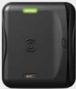
Model MTMS15 aptiQ multi-technology single gang magnetic stripe reader
